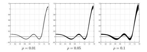
Figure 3.4: "Dream and reality," robust optimal design: samples of 100 actual diagrams for different uncertainty levels. Dotted line: the target diagram.
