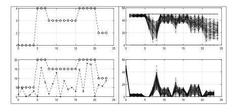
Figure 3.5: Left, top: hourly pumping cost. Left, bottom: upper bounds  $\overline{d}_t$  on hourly demands (o) and sample demand trajectory (+). Right: 100 sample level (top) and control (bottom) trajectories. Pay attention to how close to the tank's capacity are tank levels in the first five  $(1 \le t \le 5)$  "cheap pumping – low demand" hours and to how intensive is the pumping in the beginning (t = 0).
